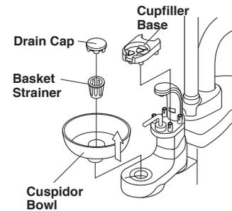
Fig.5-1 Cuspidor Bowl, Drain Cap and Basket Strainer
