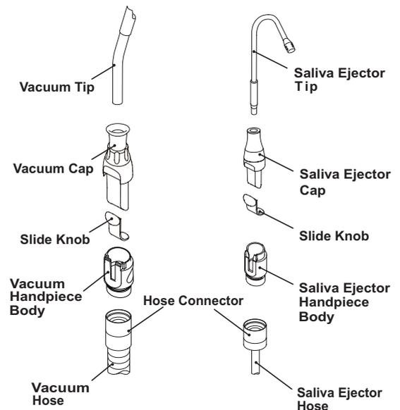
Fig.5-3 Vacuum Handpiece and Saliva Ejector Handpiece
