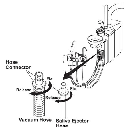
Fig.5-7 Vacuum and Saliva Ejector Hose
