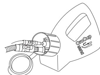
Fig.5-6 Cleaning Vacuum /Saliva Ejector Lines
