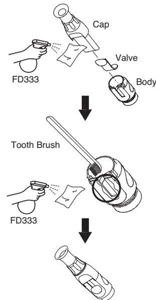
Fig.5-4 Cleaning of Vacuum Handpiece Body and Saliva Ejector Handpiece Body
