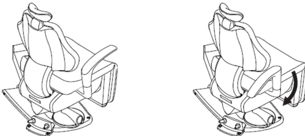
The right armrest can be rotated outward 130 degrees in a clockwise direction.
