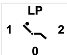
Momentarily depress **1** the auto mode stick switch to left side, the chair will move to the preset-1 position automatically.
