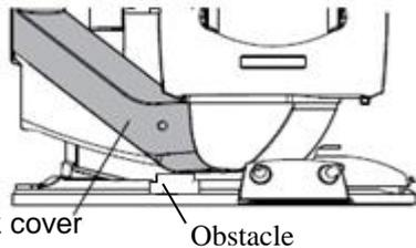
All chair movements can be stopped automatically by the safety switch function when there are any articles under roll up legrest. In that case, only seat lifting and backrest rising can be operated.
