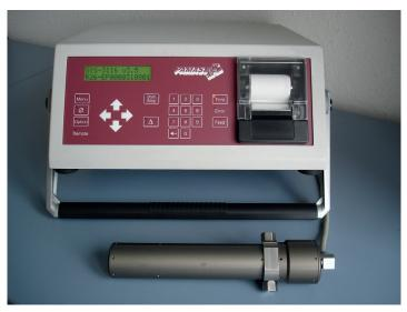
Integrated in the Floc Size Analyser PAMAS FSA-2002 are the particle counter PAMAS 3116 and the light extinction sensor PAMAS HCB-LD-900. Advanced PAMAS sensor technology guarantees highest measuring accuracy and statistical reproducibility of the measuring results.
