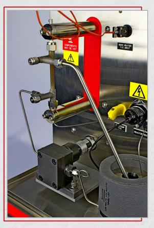
The TEOST<sup>™</sup> 33C method has indicated that deposit-formation in the turbocharger is additive-sensitive (additive-free refined mineral base oils of relatively high paraffin content form little deposits by themselves in the TEOST<sup>™</sup> 33C). The test has become a required standard for engine oils by OEMs.
