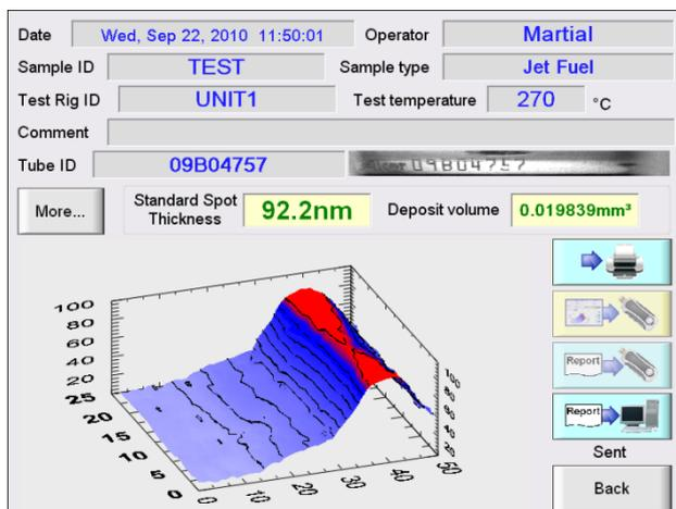
The DR10 measures the deposit thickness around the surface of the tube. At the end of the test, it displays in SI units a 3D mapping of the deposit formed along and around the whole length of heater tube. In addition the instrument reports average and maximum thicknesses and total volume deposit.
