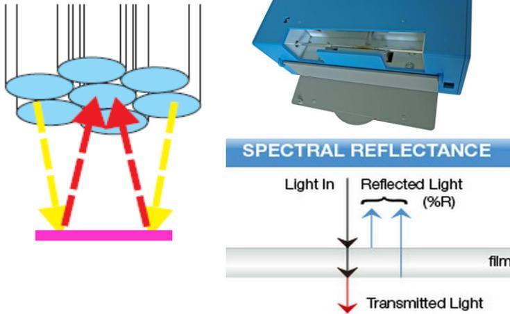
The reflected light is collected and the light interference created by the deposit is processed by a spectrometer. The software analyzes the interference fringes and calculates the deposit thickness.
