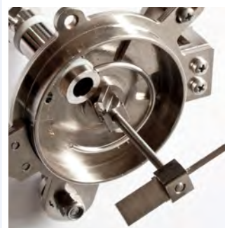
Dual flash point detection system: by ionisation ring, by thermal sensor.
