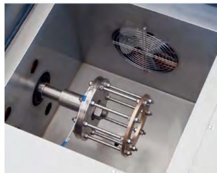
Newlab 800: Low-temperature Torque, testing chamber. Best raw materials and simplicity in construction, strong points that make it appreciated.
