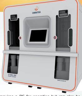
The U-VIsc requires a PC for operation but can also be controlled as a stand-alone unit through the responsive color touch screen interface. For data collection, storage, calculations and reporting, an advanced PC software application is provided with the instrument, which can gather data from up to 4 instruments simultaneously.
