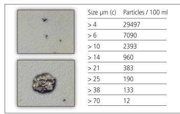
More than just providing the triple code according to ISO 4406, PAMAS S50P AVTUR measures the particle number in eight different size channels and early alerts in case of failures caused by bigger particle sizes (e.g. corrosion).
