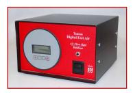
The use of an exit air device is required in D892 to measure the total air volume that has passed through each gas diffuser during the 5-minute blowing period — unless the operator choses to run according to the Alternative Procedure per Section 11 of the D892 method. The Tannas Digital Exit Air Device is the best alternative for this measurement. Tannas also offers a more basic Inverted Cylinder device at a lower price point. Contact us for details.
