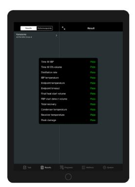
"Pass / Fail" test validation helps operators process only those results that are obtained from correctly executed tests. The validation is based on pre-defined method limits such as "Time to IBP", "IBP/FBP temperature", "Condenser/receiver temperature", distillation rate, etc.
