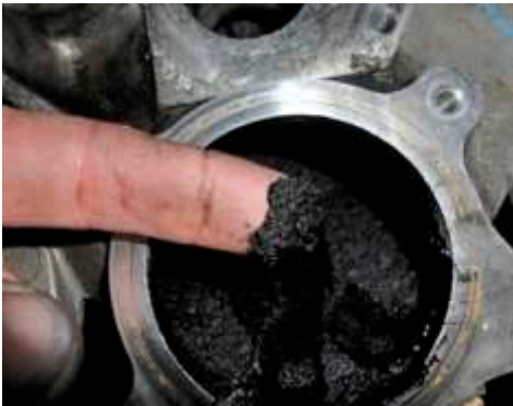
Example of extreme soot build up
