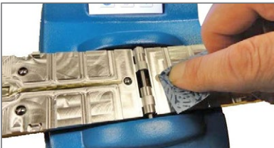
Open the two parallel plates for easy cleaning.
