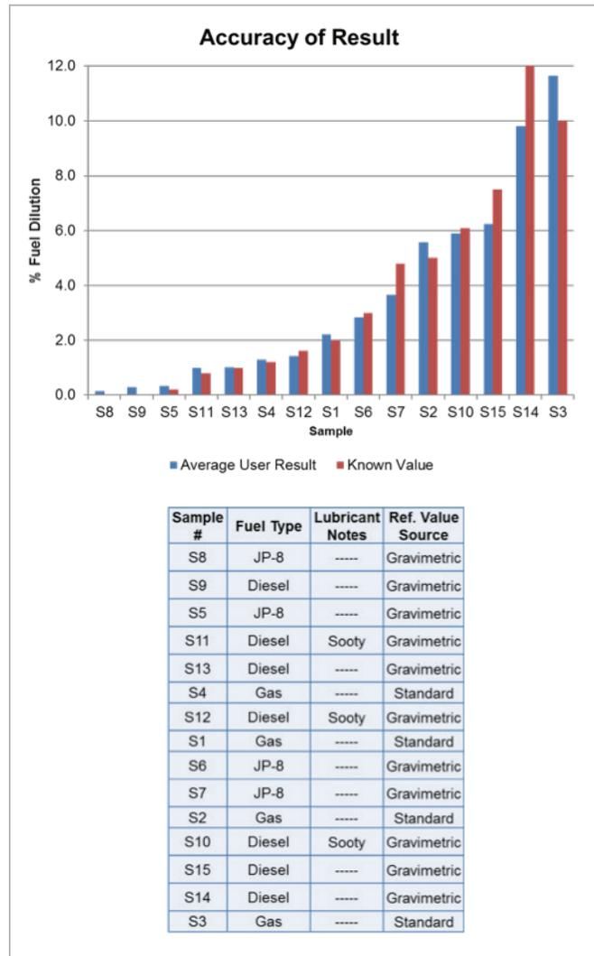
**Figure 10:** Average user result compared to the known reference value for each test sample.
