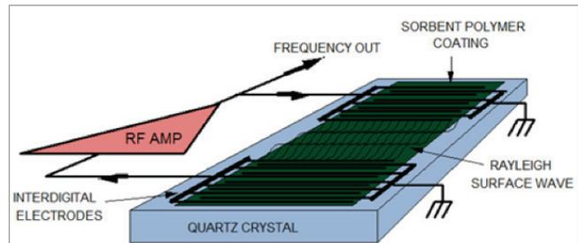
Figure 4: SAW sensors capture the response of a species specific coating and convert it to an electrical signal of equal magnitude.
