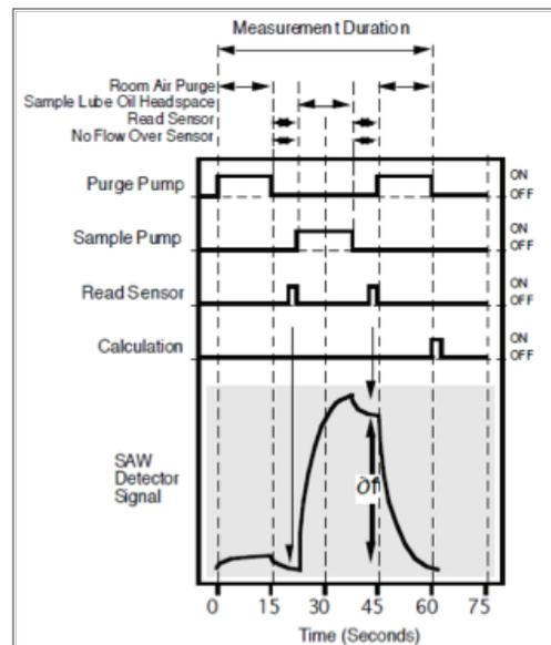
Figure 5: Typical measurement cycle and response time for fuel dilution meter
