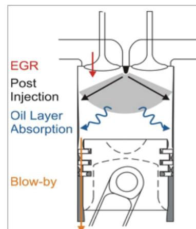
**Figure 1:** Sources of excess fuel in engine lubricants are EGR (exhaust gas recirculation, post injection (late) cycle, oil layer absorption and blowby past the
