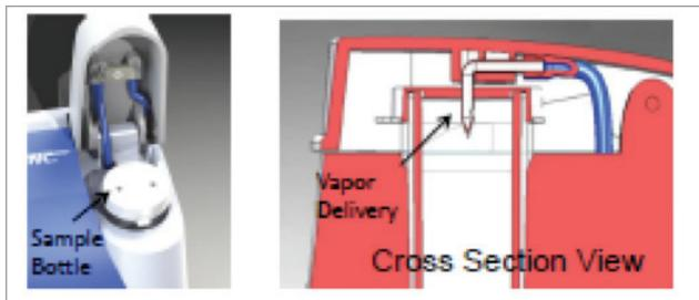
Figure 8: New headspace design improves repeatability and lowers risk of fuel carryover into sensor
