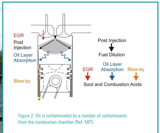
Figure 2: Oil is contaminated by a number of contaminants from the combustion chamber (Ref: MIT)
