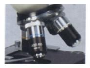
Achromatic parfocal objectives, the x40 and x100 (oil) are spring loaded for slide safety.
