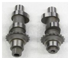
These Andrews 26N bolt-in cams fit 88–95 inch TC with stock compression ratio, and are great for two-up touring.
