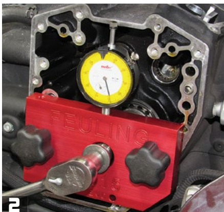
2 Dan uses Feuling tool #9015 fitted with a dial indicator to check the pinion shaft's runout to ensure the fly-wheel assembly is within Feuling's (0.025") and H-D's (0.012") usable limit. Our runout is 0.002".
