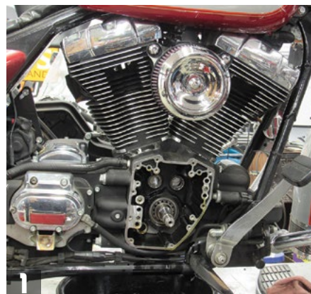
Here's our 2005 Electra Glide up on Dan's lift with the right side cover, front right floorboard, both saddlebags, and entire exhaust system removed. The gearcase compartment has also been emptied, and the lifters, pushrods, and pushrod tubes are also removed.
