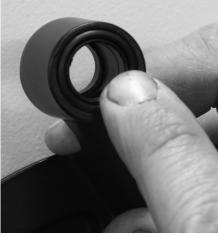
Dan inserts a new Ness O-ring into each of their grooves in the Ness backing plate. The O-rings go in dry, but you can put a small dab of silicone on them to hold them in place if needed.
