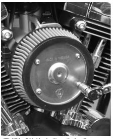
With a little blue Loctite on the four Nesssupplied screws, Dan attaches the Ness filter element to the backing plate using a 5/32" Allen. He then torques all four bolts to 36-60 in-lbs.
