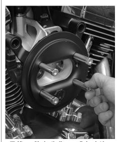
After positioning the Ness-supplied gasket between the Ness backing plate and throttle body, Dan threads in the four Ness standoffs.
