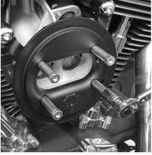
Dan can now torque the four Ness standoffs to 36–60 in–lbs. using a 1/2" socket.
