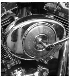
The owner wanted to reinstall the stock air cleaner cover, which goes on with a little blue Loctite on the stock bolt's threads. Dan uses a 5/16" Allen to torque the bolt to 36-60 in-lbs. MB
