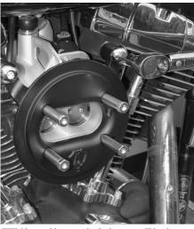
After making sure the 0-rings are still in place, Dan threads in both Ness-supplied breather bolts, with a little blue Loctite on their threads. He torques them to 10-12 ft-lbs. using a 5/16" Allen.
