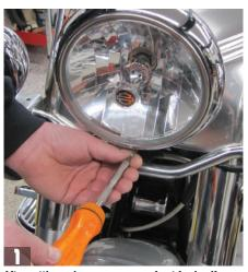
After putting a clean rag over your front fender, if you choose, remove the screw that holds the trim ring using a #2 Phillips screwdriver. Put the ring and screw aside for reinstallation later on.
