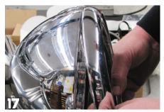
There are two tabs on the top of the stock headlight bucket that have a small black plastic collar on them. Align these two tabs with the two slots in the top inner face of the headlight trim ring.
