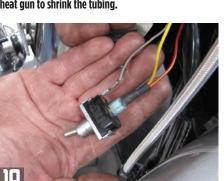
Plug the new connector onto the back of the switch. Make sure it's secure. Then reinstall the switch in the left triple tree cover.
