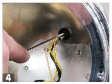
Poke a 1/8"-diameter metal rod (clothes hanger) through the grommet in the housing to open it up and make room for the wire you need to thread through it next. Coating the rod with a little dielectric grease will help.
