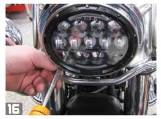
Now reinstall the stock beauty ring using the three stock screws and a #2 Phillips screwdriver.
