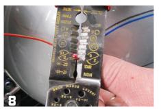
Using wire strippers, bare about 3/8" of the 16-gauge wire you just ran. Also use wire cutters to remove the blade connector from the stock wire you just pulled from the spotlight switch and bare about 3/8" of that wire.
