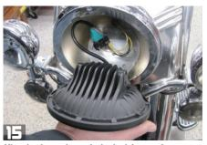
Align the three tabs on the back of the new Cyron headlight to the three notches in the stock headlight bucket.
