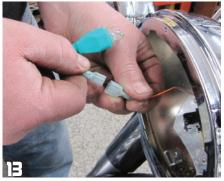
Join the two connectors you just installed. Some people like to then wrap some electric tape over the two connectors.
