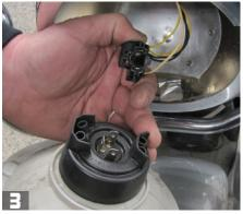
Disconnect the headlight harness from the back of the stock headlight. (The headlight will not be reused.) If you don't want to connect the daytime running lights, jump to step 14.
