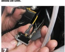
Pull the yellow wire (the one that's activated when this switch is turned on) from the back of the switch.
