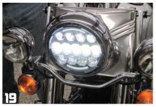
Turn on the ignition and check the low and high beams to make sure they work. Check the top and bottom daytime running lights if you opted to activate them. **AIM**
