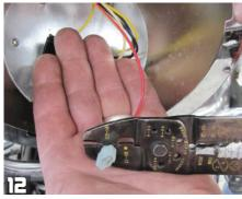
Cut the wire you installed so about 7" of it is in the headlight bucket and bare about 3/8" of the wire. Then install a female blade connector on the wire and a male connector onto the short red wire on the new LED headlight plug.
