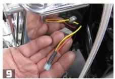
After twisting the two wires together, slip a 1" length of heat shrink over the wires. With a crimping tool, put a new blade connector onto the wires and then use a heat gun to shrink the tubing.
