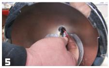
Now poke an 18" length of 16-gauge wire though the rubber grommet and route it out of the left side of the triple tree covers.
