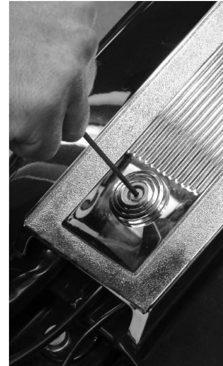
19 After securing the dash's bottom using the stock bolt and a Phillips screwdriver (ours has a decorative washer and special bolt), Dan tightens the nut, refills the tank and verifies that everything works. MB
