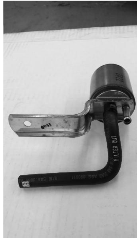
8 To set up the fuel filter (#61343-95), Dan slips the Filter Out end of the hose (#62358-95) onto the fitting closest to the filter support. He then crimps on a new clamp.
