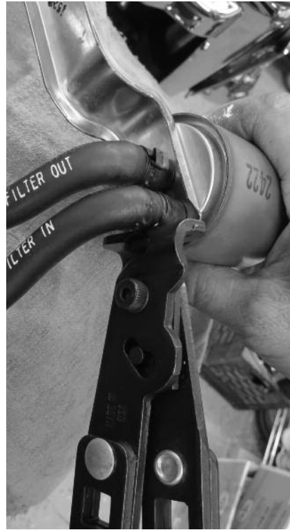
9 After slipping a new clamp onto the Filter In end of the hose from the fuel pump, Dan secures this hose to the other fitting on the fuel filter using another clamp and the crimping tool.
