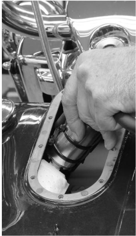
6 Dan installs the pump into the tank, over the rods, and into the tray. He then pulls the wires out of the opening in the tank and routes the hose over to the right side of the tank.
