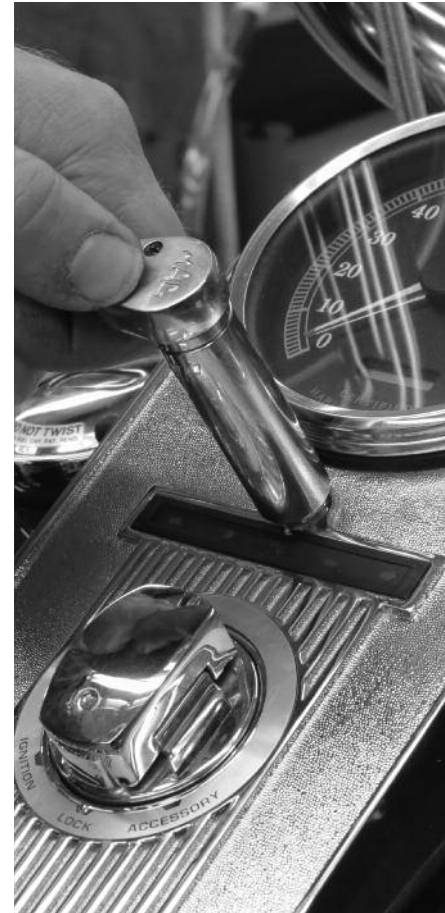
18 After making sure the rubber strip is properly positioned around the base of the dash, Dan loosely reinstalls it onto the tank using the stock nut and a 1/2" socket.
