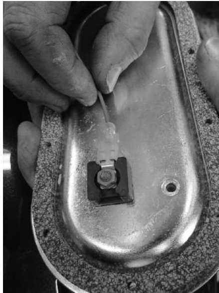
13 After making sure the tank opening is clean, Dan connects the fuel pump's red wire to the connector on the inner face of the top plate.
