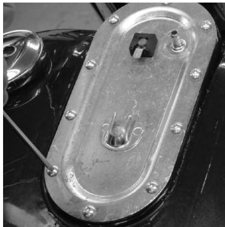
14 With a new cork gasket on the tank, Dan reinstalls the stock top plate using 10 new bolts and a T20 Torx. He torques the bolts to 36-60 in-lbs.
