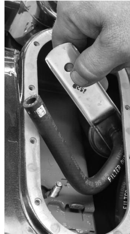
10 This is how Dan has to orientate the fuel filter assembly to get it into (or out of) the fuel tank.
