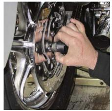
After cocking the wheel slightly sideways in the swingarm, he positions the short right wheel spacer between the wheel and rear brake caliper.
