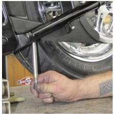
After dropping the bike down from the bike jack, he uses the H-D belt tension gauge (#HD-35381) to check the rear belt deflection. Ours is still correct even after changing out the rear wheel and pulley.
