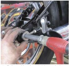
Dan positions the stock right rear wheel adjuster collar on the axle and next to the adjuster. He then sends the stock axle through the adjuster, frame, spacers, and wheel using a plastic hammer.
