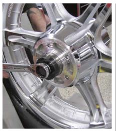
With the rear wheel in a lift's wheel chock, he uses a wheel bearing installation tool to install a wheel bearing (both the same) from the H-D installation kit into the right (primary) side of the wheel, as indicated by the lines on the wheel hub.
