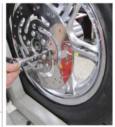
With blue Loctite on the new chrome H-D rotor bolts, he installs the new polished H-D rear brake rotor onto the new 6-Spoke wheel using a T-45 Torx. He torques the bolts to 40 ft-lbs. in a crisscross pattern.
