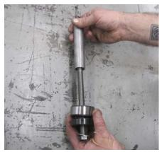
Dan slips the new wheel bearing and the proper center wheel spacer (spacer C #43608-00 for our application), both from the H-D installation kit, onto the shaft of his wheel bearing installation tool.
