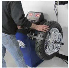
Dan can now balance the wheel on the Rob's Dyno Service spin balancing machine. He then jacks up the rear of the bike and removes the stock rear wheel from our 2006 Fat Boy. He also removes the brake pads from the rear caliper.
