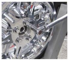
With red Loctite on the new chrome H-D pulley bolts (with washers), he installs the new chrome H-D pulley (align the pulley and wheel patterns) onto the new wheel using a 5/8" socket. He torques the bolts as per the H-D procedure.
