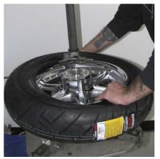
After checking the directional arrow and locating the balance dot alongside the valve stem, he installs the new Shinko 150/80-16" tire onto the H-D 6-Spoke wheel.
