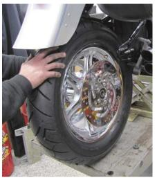
**9** Dan then positions the new rear wheel in the swingarm and wraps the rear drive belt around the pulley. He has covered the outer face of the pulley with tape to protect it and loosened the bottom belt guard hardware.
