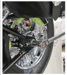
Once the axle is fully through, he reinstalls the stock left rear wheel adjuster collar on the axle, followed by the stock flat washer and nut, using a 15/16" socket. He just snugs the nut for now.
