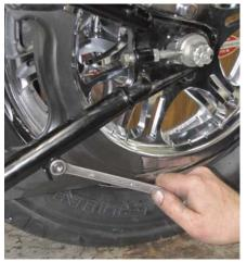
After torquing the rear axle nut to 60-65 ftlbs., he retightens the lower belt guard hardware using two 1/2" wrenches. Don't forget the one buried behind the swingarm.
