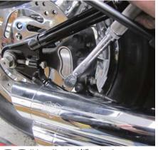
20 Using a 12-point 1/4" socket, Dan torques the two stock caliper brake pad bolts to 180-200 in-Ibs. He then checks the operation of the rear brake system. You'll have to pump the rear brake a few times to get it back to normal.
