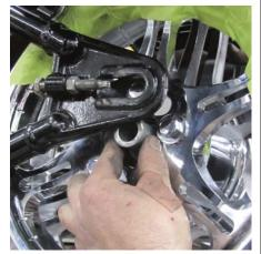
He places the long left wheel spacer between the swingarm and wheel. He then drops the bike down a little bit. He also cleans the stock axle, puts a skin coat of anti-seize on it, and sets it aside on a clean rag. pingel
