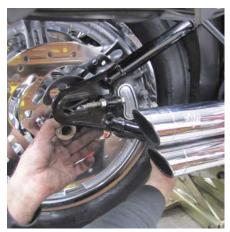
He can then position the rear brake caliper around the rear rotor with the mount section by the axle hole in the wheel.
