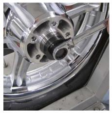
With a little oil on the edge of the new wheel bearing, he uses the bearing puller to install both the spacer and wheel bearing into the right side of the wheel.
