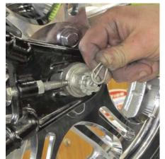
Dan then pops in the stock rear axle nut clip using a plastic hammer. If you had to move the axle adjusters to adjust the rear belt and realign the rear wheel, don't forget to tighten the lock nut on both adjusters.
