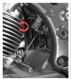
After running the Dynojet Power Commander V (PCV) harnesses (arrow) as per its instructions, Rob connects the PCV's 0<sub>2</sub> optimizers to the bike's stock 0<sub>2</sub> sensors, which no longer get connected to the stock wiring harness.
