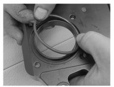
After removing the stock O-ring from the back of the stock Indian backing plate, Rob installs it onto the back of the S&S-supplied throttle body backplate.
