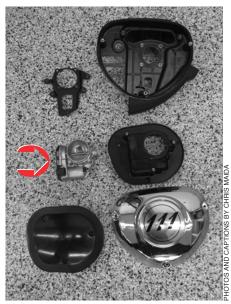
We don't normally show this, but here are all the stock parts you have to remove to install this S&S kit. The only stock part that's reused is the throttle body (arrow).
