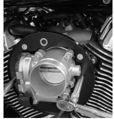
With some S&S threadlocker on the four stock throttle body bolts, Rob uses them and a 5mm Allen to secure the stock throttle body to the S&S throttle body backplate. He torques the bolts to 88.5 in-lbs.
