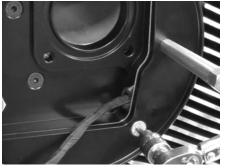
Rob uses a 4mm Allen and the last four S&S countersunk bolts, with threadlocker on their threads, to secure the S&S air filter backplate to the S&S throttle body backplate. He torgues the bolts to 88.5 in-lbs.
