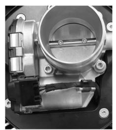
After slipping the harness into its stock clip on the throttle body, Rob reconnects it to the throttle body. (Note: to disconnect it, just squeeze the two clips on the top and bottom of the connector.)
