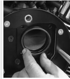
After removing the stock throttle body O-ring from the stock Indian backing plate, Rob installs it into its groove in the front of the S&S throttle body backplate.
