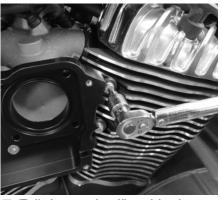
He then uses a 4mm Allen and the other two prepared bolts to secure the S&S-supplied throttle body backplate to the engine. He torques both bolts to 88.5 in-lbs.
