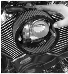
Rob now positions the S&S-supplied air filter element onto the S&S air filter backplate. He makes sure the element sits in its groove in the backplate.
