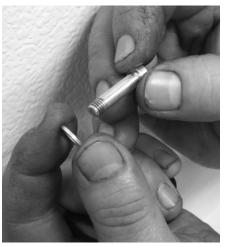
After putting a little of the S&S-supplied threadlocker onto the threads of the four S&S-supplied bolts, Rob slips one of the four S&S-supplied flat washers onto each bolt. our 2015 Roadmaster test bike, we went with the chrome S&S Nostalgic Script cover (#170-0239/\$129.95), which looks perfect with the polished engine and chrome primary cover.
