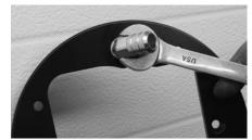
After putting some Teflon sealant onto the threads of the S&S-supplied 45-degree elbow fitting, Rob uses a 5/8" open-end wrench to install the fitting onto the S&S throttle body backplate. Note how it is orientated on the backplate.
