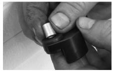
• Next in are the four S&S-supplied steel spacers, which go into the four rubber grommets he just installed.
