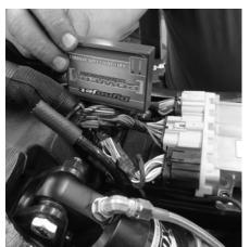
After hooking up all its connectors, Rob tucks the Dynojet Power Commander V module out of the way under the seat.
