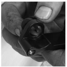
Rob then inserts the four S&S-supplied rubber grommets into their openings in the kit's backplate bracket (shown) and throttle body backplate using just his fingers. Use a little soapy water if the grommets are hard to get in.
