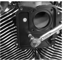
Rob uses a 4mm Allen and two of the S&Ssupplied countersunk bolts, with S&S-supplied threadlocker on the threads, to secure the other end of the S&S-supplied backplate to the S&S bracket on the engine. He torques both bolts to 88.5 in-lbs.
