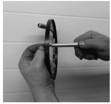
With some S&S-supplied threadlocker on the two S&S-supplied countersunk bolts, Rob secures the two S&S standoffs (hex end against the backplate) to the S&S throttle body backplate. He torques the bolts to 88.5 in-lbs. using a 4mm Allen and 1/2" wrench.
