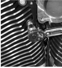
He then uses a 4mm Allen and two of the prepared bolts to secure the S&S-supplied backplate bracket to the engine. He torques both bolts to 88.5 in-lbs.
