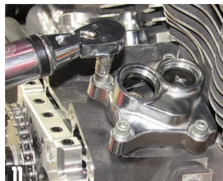
With new Feuling-supplied Comet gaskets in place, Dan reinstalls the two stock lifter covers using the stock bolts, blue Loctite, and a 3/16" Allen. He torques the bolts to 90-120 in.-lbs. in a crisscross pattern.
