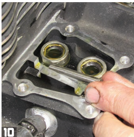
Next in are the two stock lifter anti-rotation devices, one for each cylinder's two lifters.
