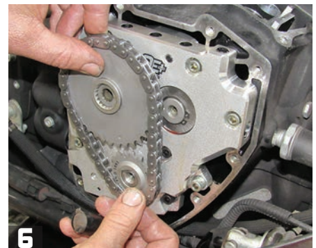
6 After he removes and positions both new Feuling sprockets in the new Feuling cam chain with their timing dots aligned, he slips both sprockets onto their shafts. They can only go on one way.
