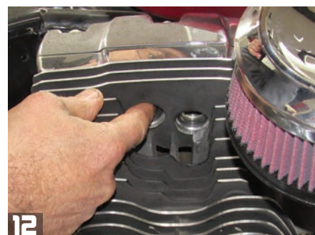
After removing the old ones, Dan installs the new Feuling-supplied Comet O-rings into the stock pushrod tubes, lifter covers, and rocker boxes. He then rotates the engine so the rear lifters are at their lowest point.
