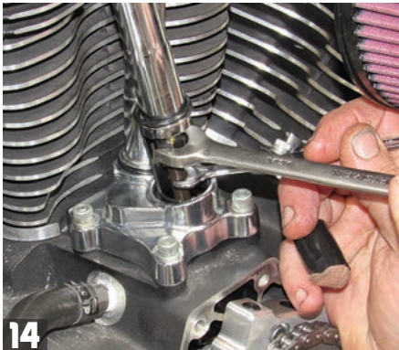
14 Using a 9/32" wrench and two 1/2" wrenches, Dan adjusts the Andrews EZ-Install pushrods as per the Andrews instructions regarding number of turns, etc. He then lets the rear lifters bleed down.
