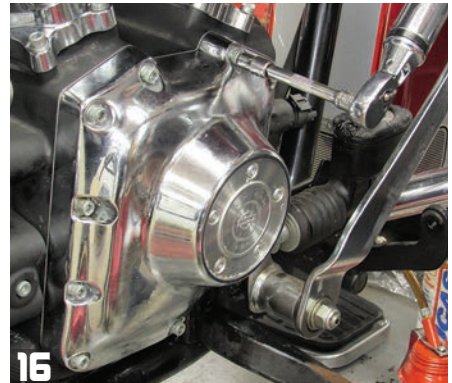
16 After putting the new Feuling-supplied Comet gasket on the right crankcase, Dan reinstalls the stock cam cover using the nine stock bolts, blue Loctite, and a 3/16" Allen. He torques the bolts to 90-120 in.-lbs.
