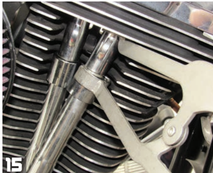
15 Once Dan has installed and adjusted the front pushrods, and has rotated the engine to check the valvetrain, he uses a special tool to pop in the stock pushrod tube retainers, but you can also use a flat-bladed screwdriver.
