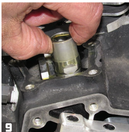
After filling the new Feuling lifters with motor oil via a pump oil can, Dan drops the new lifters into their bores in the right crankcase with their flat sides towards the front and rear wheels.
