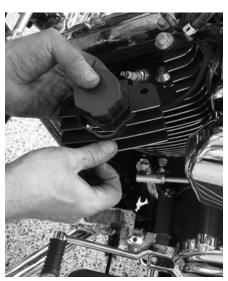
Back at Rob's shop, Dan is positioning a set of **ACCEL Stealth Super Coils over our 2014 Street** Glide's spark plugs.
