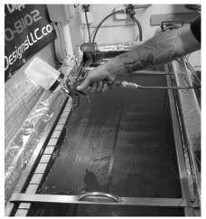
After the film is hydrated. Jim sprays on the activator, which dissolves the coating that held the paint pattern to the film. This activator will also bond the paint to the just-painted saddlebag lid.
