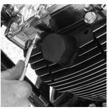
It only takes a couple of bolts and a few wires to install each ACCEL Stealth Super Coil. This setup puts a coil right on top of each spark plug.
