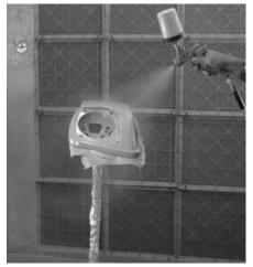
After wiping it down with a cleaner, Jim sprays on the PPG primer coat. After waiting about 30 minutes for the primer to dry, Jim sprays on the PPG tan basecoat.
