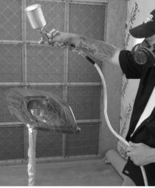
After washing and then drying the saddlebag lid, Jim sprays on the top coat of PPG clear.
