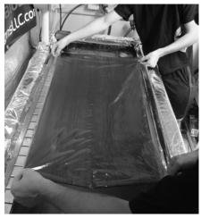
After heating the submersion tank to the proper water temperature, Jim and Blake lay the section on top of the water so there are no air bubbles under it.
