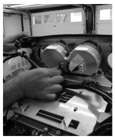
The new Dakota Digital speedo/tach gauge pack is then installed into the inner fairing and hooked to the stock wiring harness.
