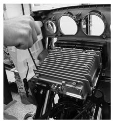
The new Harley-Davidson Stereo 6.5 GT radio upgrade is then secured into the stock radio's mount.
