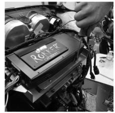
The new J&M Rokker XT Series amp is then secured to the J&M bracket, which puts it right above the H-D radio.
