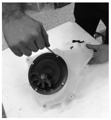
**5** Dan now installs the new J&M Rokker XT Series front speakers into the right and left stock speaker housings.
