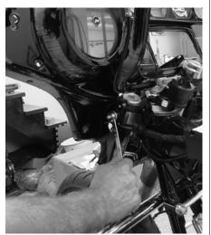
Dan now reinstalls the stock inner fairing, which has been dipped and painted by Sims Designs and Choppa J Designs, onto the bike using the stock mounts.
