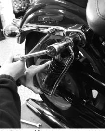
Using a 3/4" socket, Dita snugs the bolt, but she doesn't torque it just yet.
