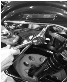
After threading the stock nut onto the end of the new bolt, Dita uses a 1/2" wrench and T-40 Torx to torque the strut cover bolt to 96-156 in-lbs. She then torques the top shock bolt to 21-35 ft-lbs.
