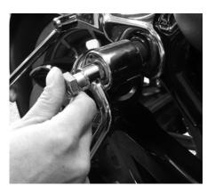
Dita inserts the bolt assembly into the top of the shock (and stock spacer, if you have one) and threads it in a little using her fingers. Use the jack to align the holes in the shock and frame if needed.
