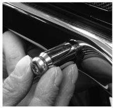
Dita then slips this bolt through the kit's chrome bracket to secure it to the fender strut cover. She threads the bolt into the strut cover all the way in.
