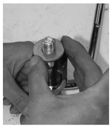
The stock large washer that was under the stock shock top cover goes on next. Dita then puts some blue Loctite on the bolt's threads if there's none on it as supplied.
