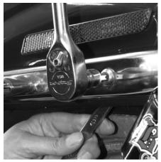
Dita uses a T-40 Torx and a 1/2" wrench to remove the fender strut support bolt. We'll reuse the stock little washer under the nut, but not the stock bolt.
