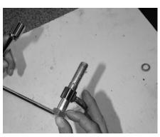
The new bolt Dita got with the H-D bracket kit goes through the chrome H-D bracket first. Make sure you have the bracket orientated correctly.
