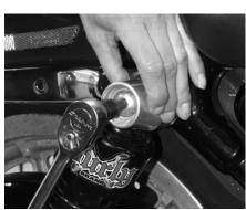
Dita removes the right rear shock's top bolt. The stock bolt and cover are not reused, but the two washers are. If your bike has a spacer between the shock and frame, you'll reuse it.
