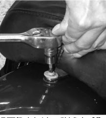
Dita also has to loosen this bolt using a T-27 Torx, so the pillion pad can be removed by pulling it back and off. You don't have to remove this bolt.
