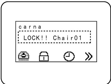
▪ When the safety mechanism is activated, the position where the safety switch is activated is displayed on the indicator.
