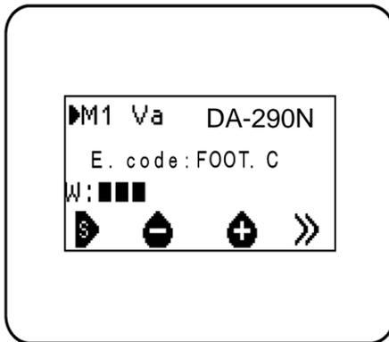
▪ The handpiece does not rotate if it is removed from the holder under the condition where you step on the foot controller pedal. At this time, the message shown on the left is displayed on the indicator, showing that the safety mechanism is activated. Be sure to pick up the handpiece first and then step on the foot controller pedal.
