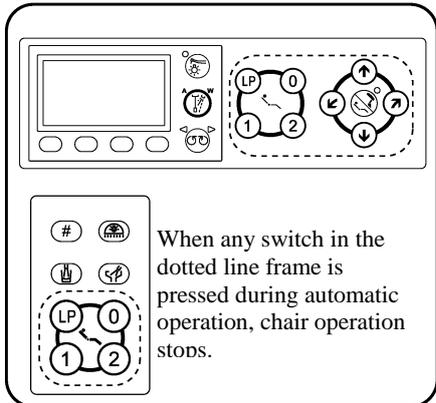
▪ The safety mechanism for stopping chair operation is activated in the following cases.
