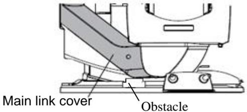
All chair movements can be stopped automatically by the safety switch function when there are any articles under roll up legrest. In that case, only seat lifting and backrest rising can be operated.
