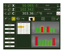
Multi edged cutter acquisition cycle: automatic recognition and measurement of each single cutting edge detected during a complete revolution of the spindle. Results are quickly visualized in a graphical format for a quick consultation or print. Possibility to select single measurement for direct positioning on the selected cutter.
