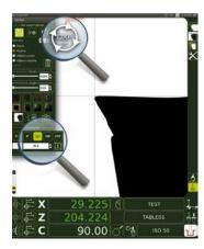
DXF profile creation fuction: automatic rotation of the tool to memorize the geometry developed and built up during full spindle rotatation to automatically generate a DXF drawing. Index function, 4 fixed position at 90°, with automatic positioning.
