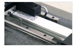
**SLIDEWAYS / OPTICAL SCALES** Elbo Controlli designed optical scales incorporated with a double rail system for the X axis movement with 3 double recirculating ball bearing sliding block grant the highest degree of accuracy. Both X & Z axes have a resolution of 1 µm.
