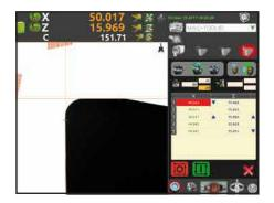
Possibility to acquire X and Z values with automatic recognition of the cutting edge. Possibility to set the measuring priority for X or Z axis. Absolute maximum measurement automatic searching with complete revolution of the spindle.
