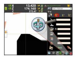
Autofocus function: all new operating mode and capability that allows the machine to measure automatically the tools, without operator presence.
