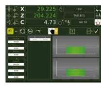
Autofocus function: automatic search and measurement for single edged tools. Possibility to acquire X, Z or both values with recognition of whether the measured values are out of tolerance. Absolute maximum searching with complete revolution of the spindle.
