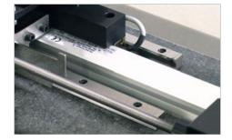
**SLIDEWAYS / OPTICAL SCALES** Custom designed optical scales incorporated with a double rail system for the X axis movement with 3 double recirculating ball bearing sliding block grant the highest degree of accuracy. Both X & Z axes have a resolution of 1 µm.
