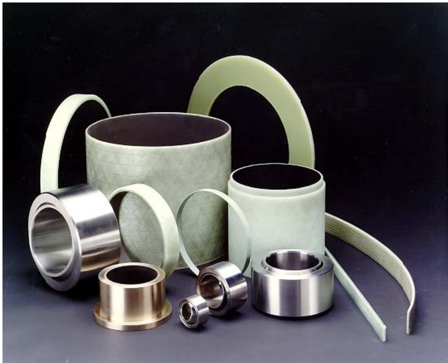
Composite bearings; filament wound, braided and laminated construction all with a KArOn liner applied are depicted above. Sleeves, thrust washers, flanged journals, guide strips and bars are shown. Glass, carbon, polyester and other fibers are combined with various resins including epoxy and polyester.
