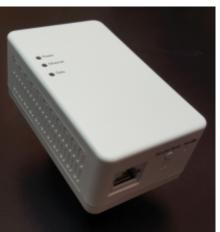
The PLS812 products family is based on the new G.hn wave2 technology, offering Gigabit Ethernet to powerline bridge – PLS812, while PLS812ac is Gigabit to powerline bridge with build in WiFi 802.11ac Access Point.
