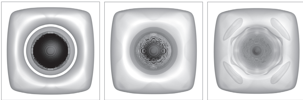
(b) Isosurfaces of \lambda_2 = -0.1 , Ra = 10^5 , \kappa = 0.25; 0; -0.25 - top view
