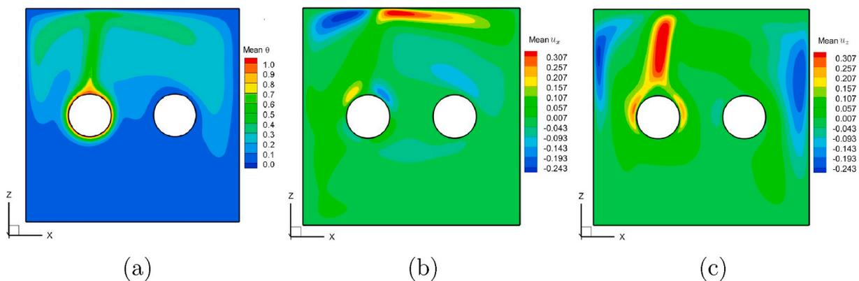
Fig. 6. Distribution of the mean flow characteristics obtained in the midplane ( $X-Z$ ) for: (a) mean temperature  $\theta$ ; (b) mean  $u_x$  velocity component; and (c) mean  $u_z$  velocity component.  $\delta = 0.4$ ,  $Ra = 6.25 \times 10^5$ . The results were obtained on a  $200^3$  structured uniform grid.
