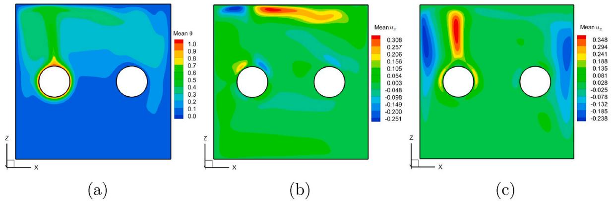
**Fig. 11.** Distribution of the mean flow characteristics obtained in the midplane ( $X-Z$ ) for: (a) mean temperature  $\theta$ ; (b) mean  $u_x$  velocity component; and (c) mean  $u_z$  velocity component.  $\delta = 0.5$ ,  $Ra = 6.25 \times 10^6$ . The results were obtained on a  $200^3$  structured uniform grid.
