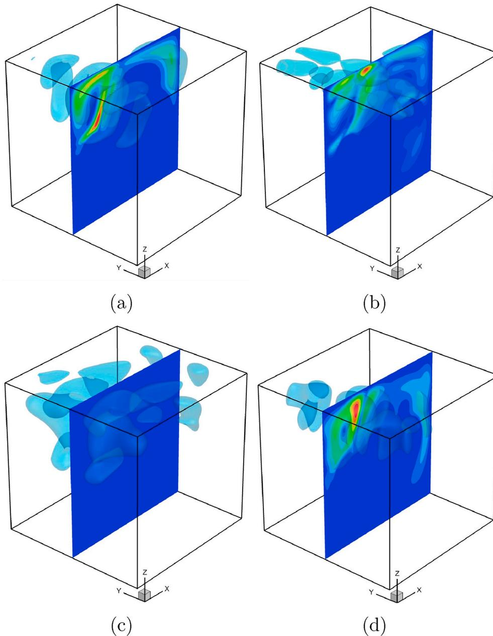
**Fig. 17.** Isosurfaces of oscillation amplitudes obtained for: (a) temperature,  $\theta$ ; (b)  $u_x$  velocity component; (c)  $u_y$  velocity component; (d)  $u_z$  velocity component. The isosurfaces confine the regions characterized by at least 25% of the absolute maximum value. Colors correspond to the relative intensity of the oscillations.  $\delta = 0.6$ ,  $Ra = 1.4 \times 10^6$ .
