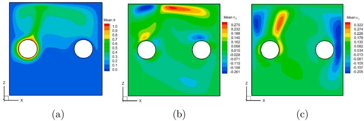
**Fig. 16.** Distribution of the mean flow characteristics obtained in the midplane ( $X-Z$ ) for: (a) mean temperature  $\theta$ ; (b) mean  $u_x$  velocity component; and (c) mean  $u_z$  velocity component.  $\delta = 0.6$ ,  $Ra = 1.4 \times 10^6$ . The results were obtained on a  $200^3$  structured uniform grid.
