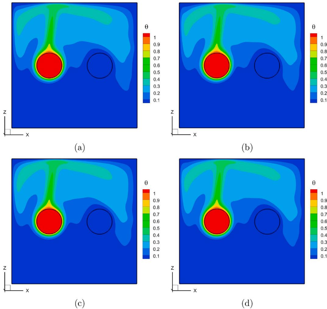
Fig. 5. Temperature distribution in the midplane ( $X-Z$ ) of the cubical enclosure obtained for 4 representative time instances of the  $\overline{Nu}_h$  time evolution as shown in Fig. 4: (a) maximal value of  $\overline{Nu}_h$  (P1); (b) intermediate value of  $\overline{Nu}_h$  (P2); (c) minimal value of  $\overline{Nu}_h$  (P3); and (d) intermediate value of  $\overline{Nu}_h$  (P4). The data was obtained for values of  $\delta = 0.4$ ,  $Ra = 6.25 \times 10^6$ .
