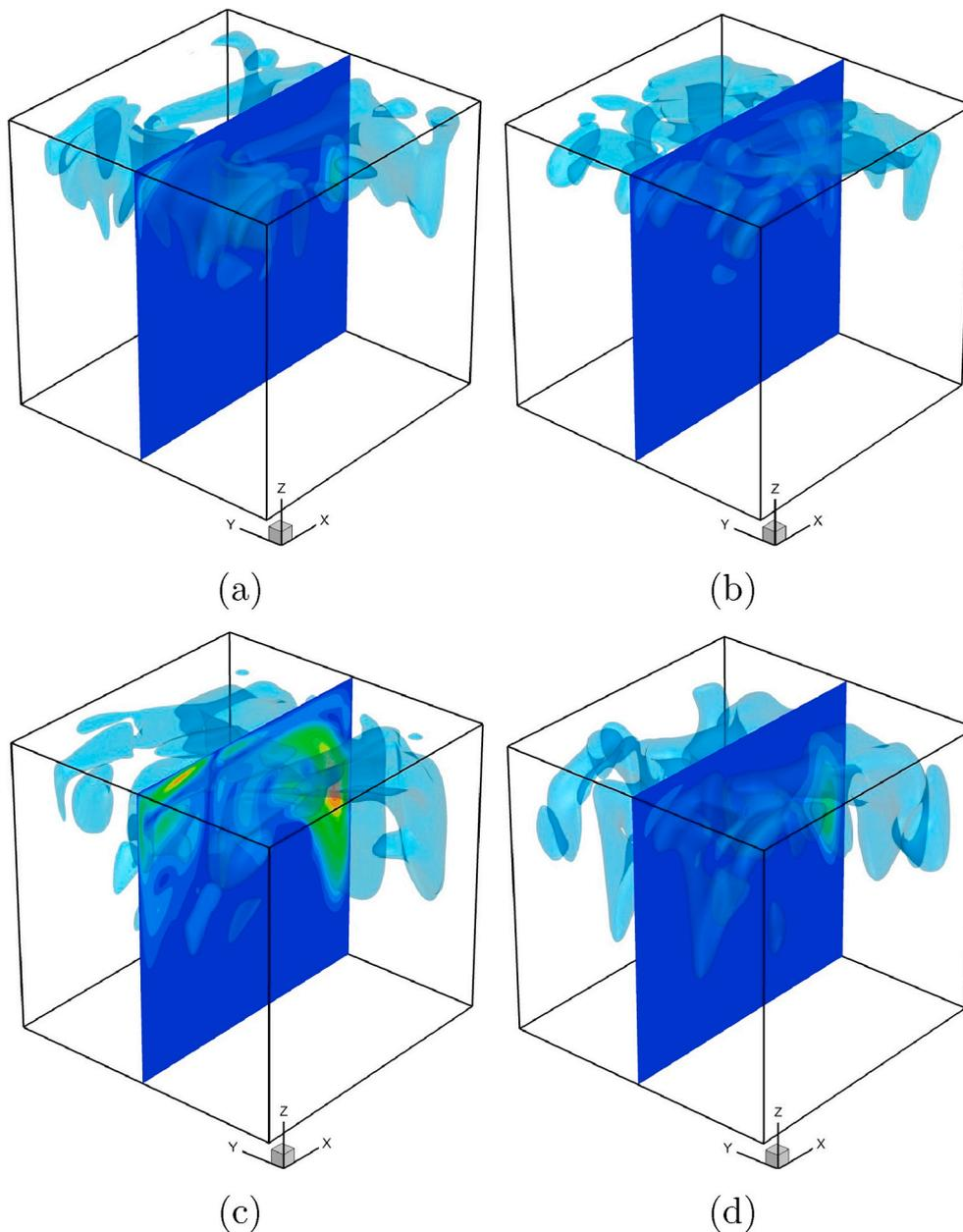
**Fig. 7.** Isosurfaces of oscillation amplitudes obtained for: (a) temperature,  $\theta$ ; (b)  $u_x$  velocity component; (c)  $u_y$  velocity component; and (d)  $u_z$  velocity component. The isosurfaces confine the regions characterized by at least 25% of the absolute maximum value. Colors correspond to relative intensity of the oscillations.  $\delta = 0.4$ ,  $Ra = 6.25 \times 10^6$ .
