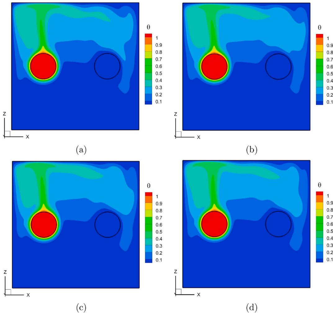
Fig. 10. Temperature distribution in the midplane ( $X-Z$ ) of the cubical enclosure obtained for 4 representative time instances of the  $\overline{Nu}_h$  time evolution as shown in Fig. 9: (a) maximal value of  $\overline{Nu}_h$  (P1); (b) intermediate value of  $\overline{Nu}_h$  (P2); (c) minimal value of  $\overline{Nu}_h$  (P3); and (d) intermediate value of  $\overline{Nu}_h$  (P4). The data was obtained for the values of  $\delta = 0.5$ ,  $Ra = 6.25 \times 10^6$ .
