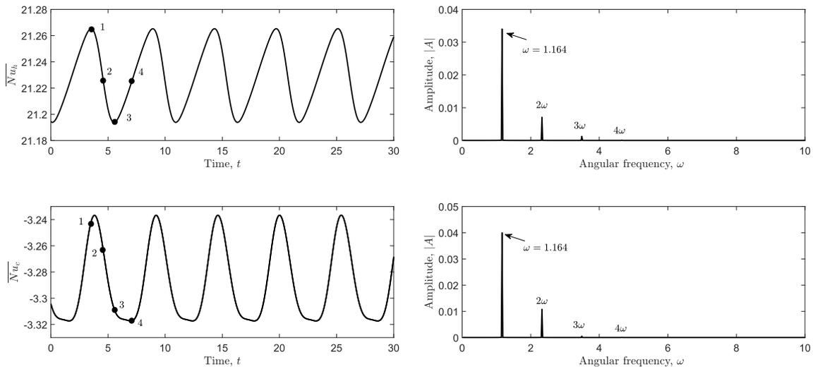
Fig. 14. Time evolution of the averaged  $\overline{Nu}_h$  and  $\overline{Nu}_c$  numbers and the corresponding Fourier spectra obtained for the values of  $\delta = 0.6$ ,  $Ra = 1.4 \times 10^6$ .
