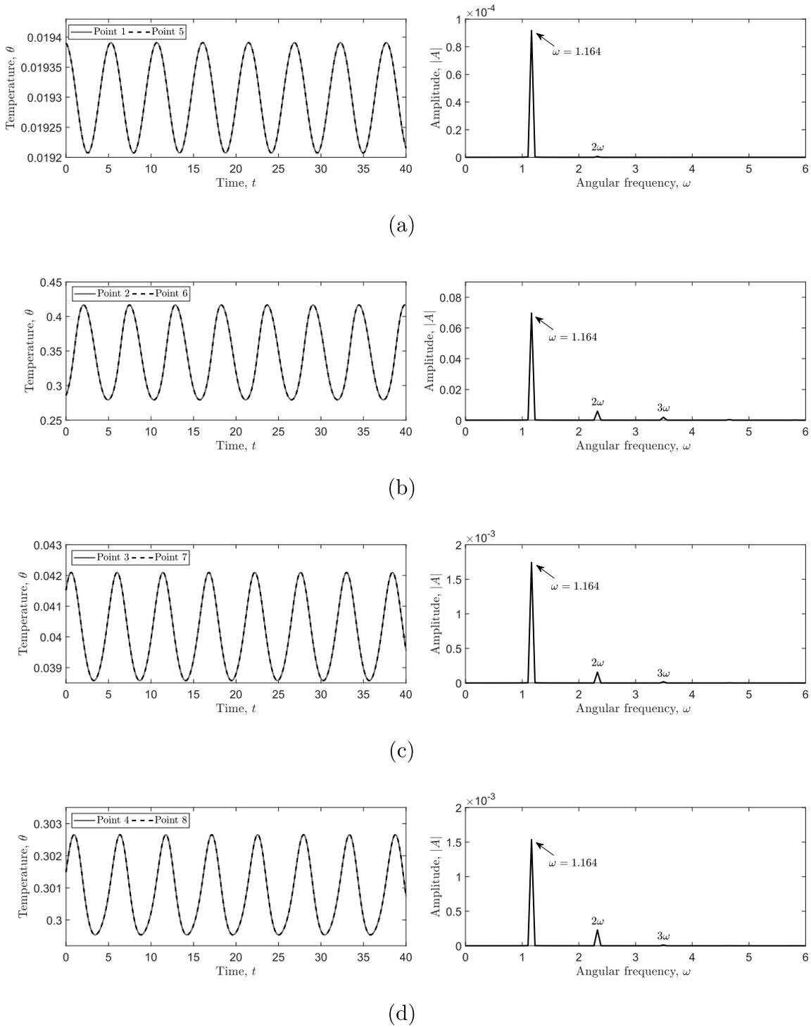
**Fig. 18.** Time evolutions and Fourier spectra monitored at four pairs of points symmetrically distanced relative to the ( $X-Z$ ) midplane for  $\delta = 0.6$ ,  $Ra = 1.4 \times 10^6$ : (a) P1 and P5; (b) P2 and P6; (c) P3 and P7; (d) P4 and P8. The results were obtained on a  $200^3$  structured uniform grid.
