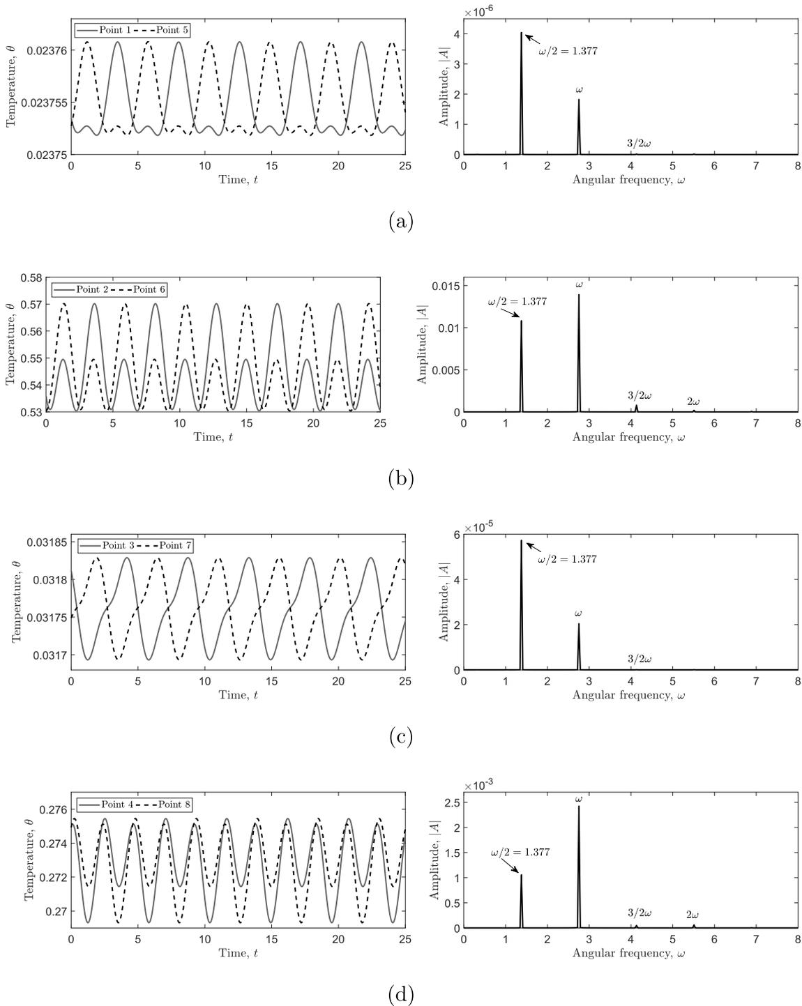
**Fig. 13.** Time evolutions and Fourier spectra monitored at four pairs of points symmetrically positioned relative to the  $(X-Z)$  midplane for  $\delta = 0.5$ ,  $Ra = 6.25 \times 10^6$ : (a) P1 and P5; (b) P2 and P6; (c) P3 and P7; (d) P4 and P8. The results were obtained on a  $200^3$  structured uniform grid.
