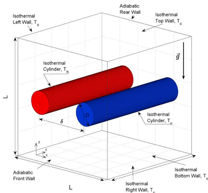
**Fig. 1.** Physical model of a tandem of hot and cold cylinders horizontally aligned inside a cold cube.
