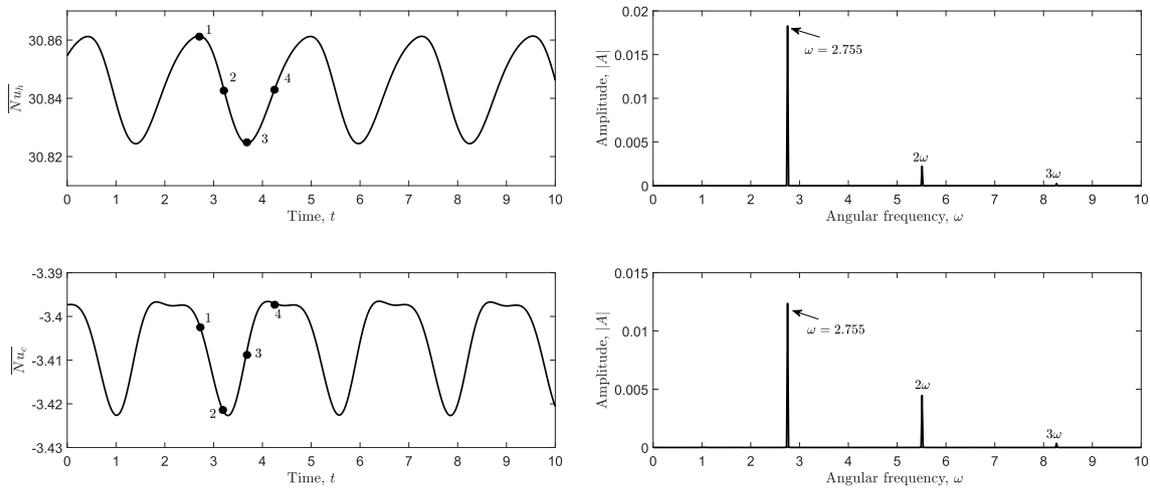
Fig. 9. Time evolution of the averaged  $\overline{Nu}_h$  and  $\overline{Nu}_c$  numbers and the corresponding Fourier spectra obtained for the values  $\delta = 0.5$ ,  $Ra = 6.25 \times 10^6$ .
