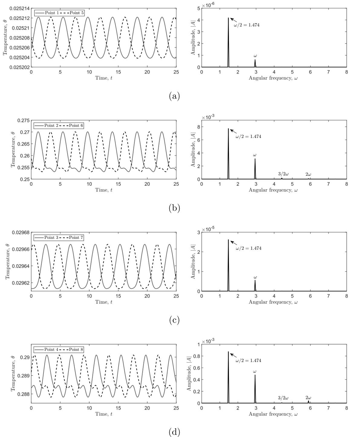
**Fig. 8.** Time evolutions and Fourier spectra monitored at four pairs of points symmetrically positioned relative to the ( $X-Z$ ) midplane for  $\delta = 0.4$ ,  $Ra = 6.25 \times 10^6$ : (a) P1 and P5; (b) P2 and P6; (c) P3 and P7; (d) P4 and P8. The results were obtained on a  $200^3$  structured uniform grid.
