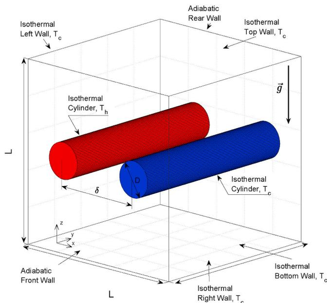
**Fig. 1.** Physical model of a tandem of hot and cold cylinders horizontally aligned inside a cold cube.
