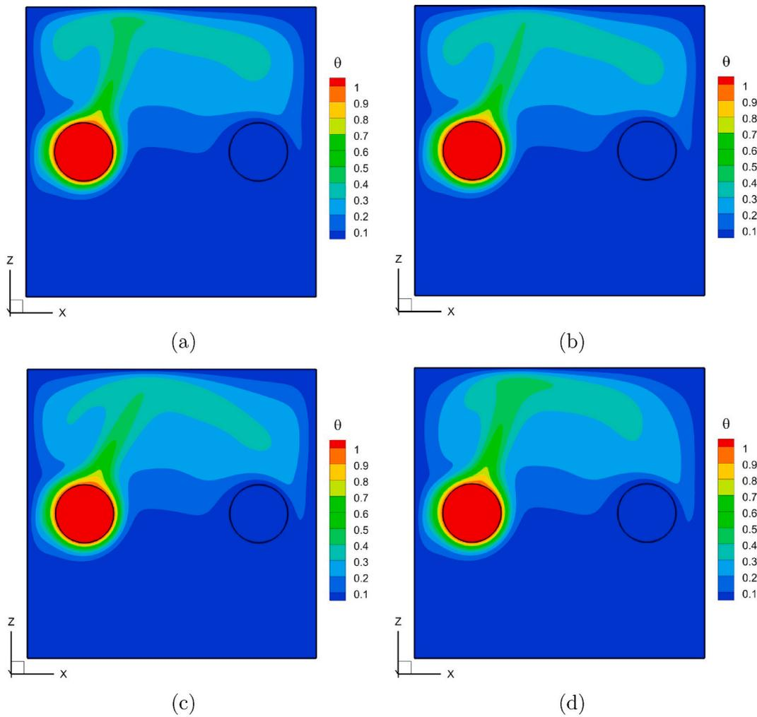
Fig. 15. Temperature distribution in the midplane ( $X-Z$ ) of the cubical enclosure obtained for 4 representative time instances of the  $\overline{Nu}_h$  time evolution as shown in Fig. 14: (a) maximal value of  $\overline{Nu}_h$  (P1); (b) intermediate value of  $\overline{Nu}_h$  (P2); (c) minimal value of  $\overline{Nu}_h$  (P3); and (d) intermediate value of  $\overline{Nu}_h$  (P4). The data was obtained for the values of  $\delta = 0.6$ ,  $Ra = 1.4 \times 10^6$ .
