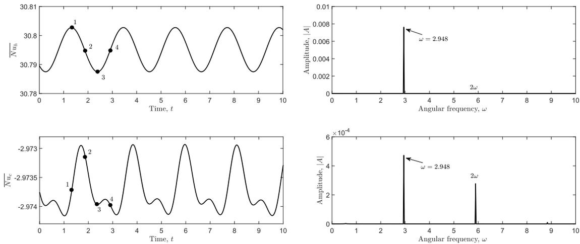
**Fig. 4.** Time evolution of the averaged  $\overline{Nu}_h$  and  $\overline{Nu}_c$  numbers and the corresponding Fourier spectra obtained for the values of  $\delta = 0.4$ ,  $Ra = 6.25 \times 10^6$ .
