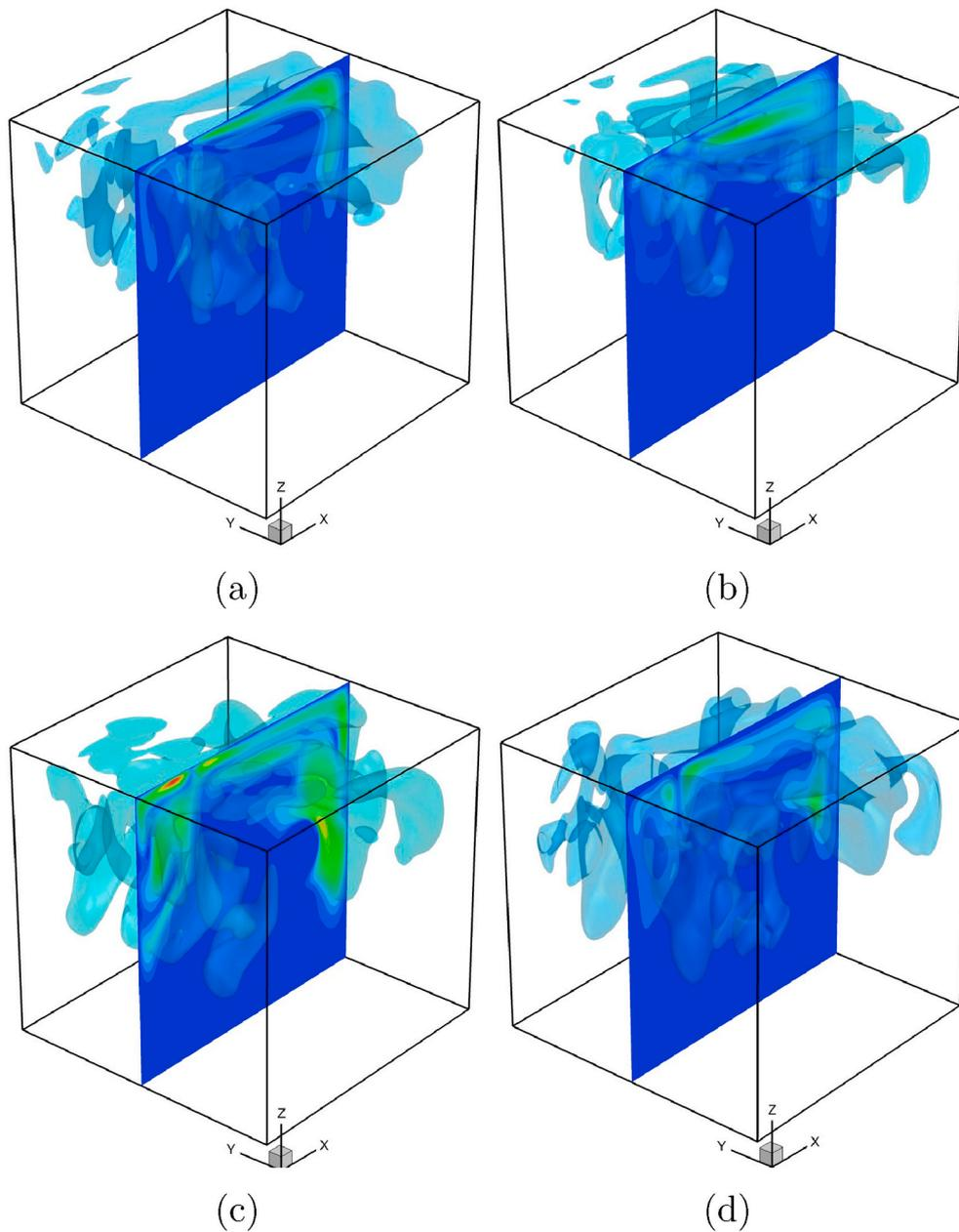
**Fig. 12.** Isosurfaces of oscillation amplitudes obtained for: (a) temperature,  $\theta$ ; (b)  $u_x$  velocity component; (c)  $u_y$  velocity component; and (d)  $u_z$  velocity component. The isosurfaces confine the regions characterized by at least 25% of the absolute maximum value. Colors correspond to the relative intensity of the oscillations.  $\delta = 0.5$ ,  $Ra = 6.25 \times 10^6$ .
