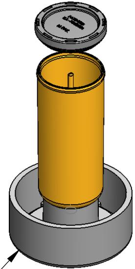
SPECIAL PUCK FOR FILLING AND CAPPING. THIS PUCK PREVENTS ACTUATION OF PUMP DURING CAPPING. AVAILABLE FROM PCA
