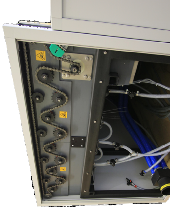
reliable chain drive system (no worm gears are used !)
