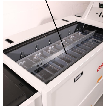
# anti oxidation cover for wet section
