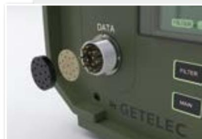
Pre-cut conductive gaskets ensure sealing and electromagnetic shielding. Gaskets are cut from sheets made in a range of conductive materials and thicknesses from 0.5 mm to 10 mm.
