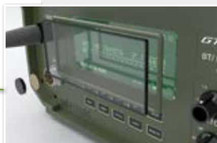
Shielded windows provide electromagnetic protection to the front face of display screens. Available in polycarbonate or glass, their light transmission can be as much as 82%.
