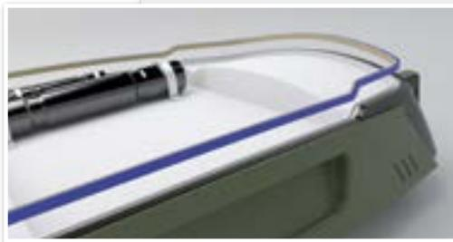
The bi-material seal is made of a conductive silicone and an insulating silicone bonded together by co-extrusion into one seal. This separates the shielding and sealing functions and the seal is, therefore, much more resistant to salt fog type extreme environments.
