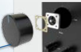
Pre-cut conductive gaskets ensure sealing and electromagnetic shielding. Gaskets are cut from sheets made in a range of conductive materials and thicknesses from 0.5mm to 10mm.
