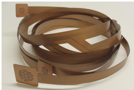
5metre (200inch) long, 6 layer flex PCB
