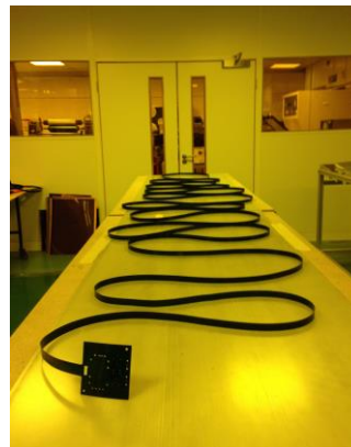
15metre, impedance controlled data harness
